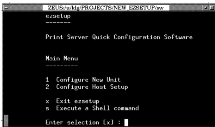
10. Enter “1” for “Configure New Unit” since you want to configure an M205/M206 with its TCP/IP settings.
